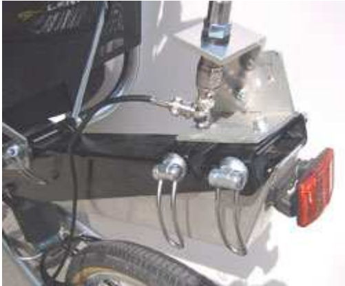
The antenna mounted on the rear frame of the bike.
