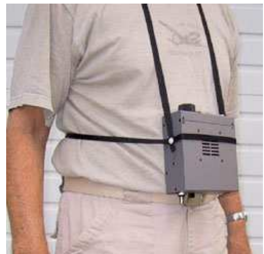
The K1 "mounted" on the author. By using your body as a mount, access to the controls is easy.
